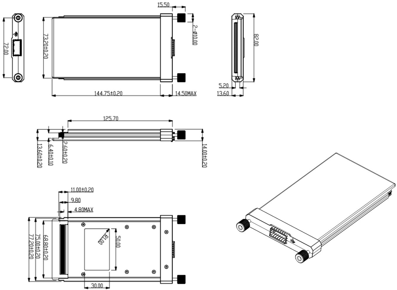
Figure4. Mechanical Specifications
