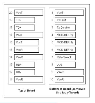
Figure3. Pin Diagram
