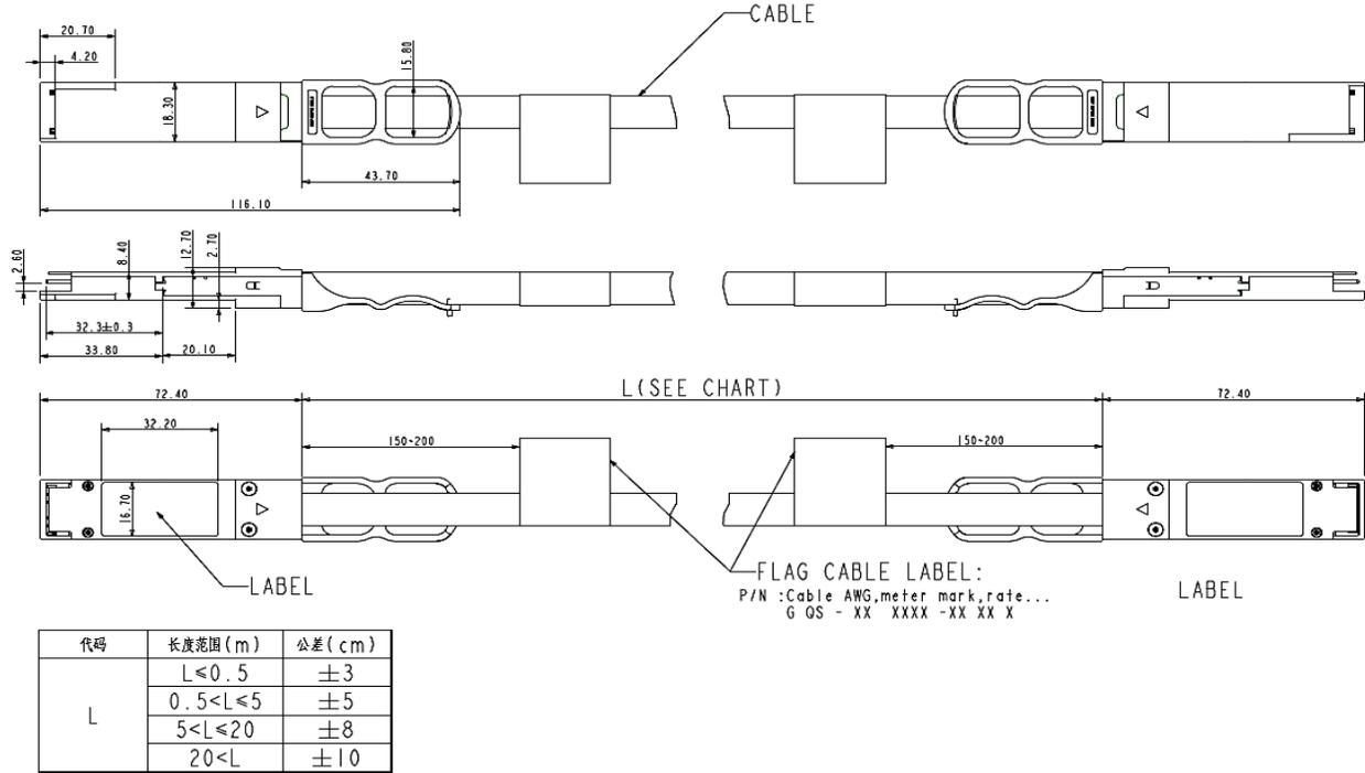
Figure2. Mechanical Specifications
