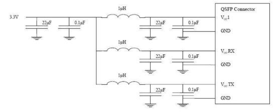
Figure 3. Host Board Power Supply Filtering
