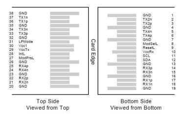
Figure 2. Electrical Pin-out Details
