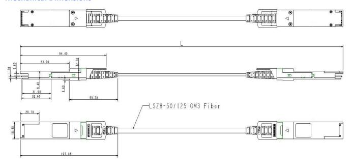
Figure 8. Mechanical Specifications
