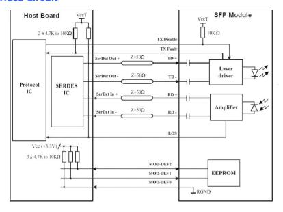
Figure 4. Interface Circuit
