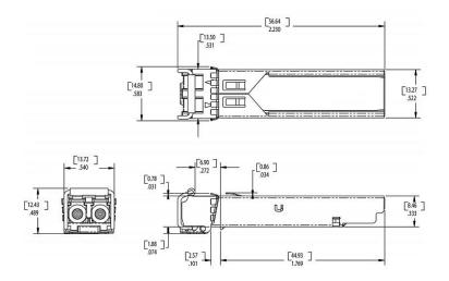
Figure 5. Mechanical Dimensions
