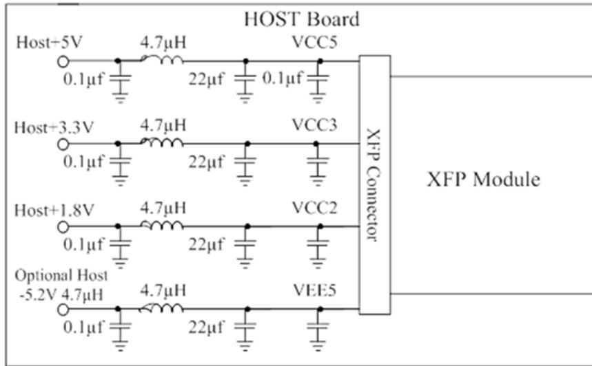
Figure 3: Recommended Host Board Power Supply Circuit
