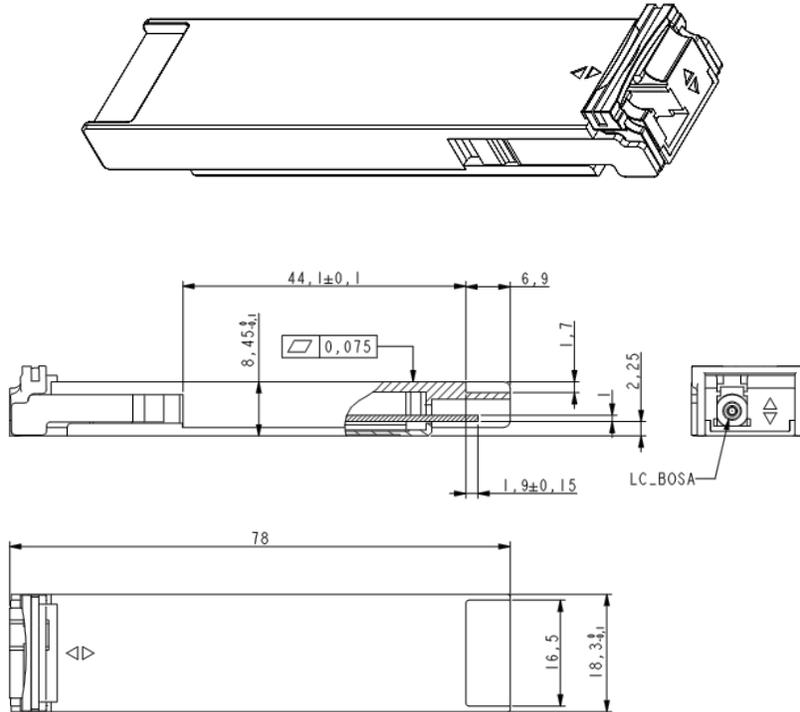
Figure5. Mechanical Specifications
